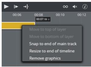
• Move to top/bottom of layer: In the event graphics are overlapping, move one graphic behind or in front of other graphics on the timeline. Graphics moved to the top will not be
