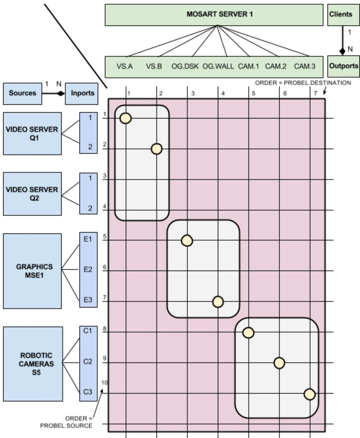
Physical devices are localized on the vertical dimension organized as *Sources* with *Inputs*. A source may have one or several *inputs*. Viz Mosart servers are localized at the horizontal dimension organized as *Clients* with *Outports*. A *client* may have one or several *outports*.
