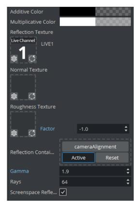
This material renders your talent into the reflection container, so this container needs to be assigned to the **Reflection Container**. In our setup this is the aligned, billboarded container named *cameraAlignment*. The source also needs to be assigned, drag the *Live1* (respective the source used) onto **Reflective Texture.**
