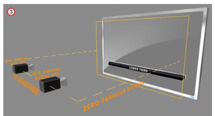
The eye separation defines how flat or deep an object shows. If the eye separation is increased, the scene shows deeper (4):
