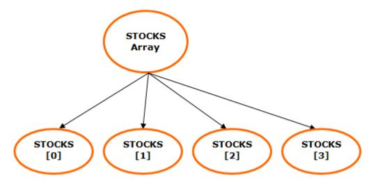
In the figure, an array of stocks of size four is shown. As can be seen each of its children are named Stocks[0], Stocks[1], and so on. To enter data to the array element number 2:
