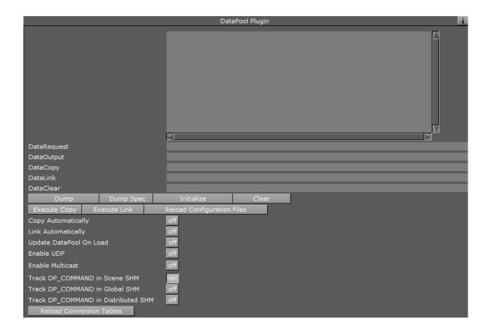
• Data: Allows the user or external software to define new DataFields and assign data to DataFields. The field content is saved with the scene when the scene is saved in Viz. Data is a text parameter. All commands/assignments should be semicolon separated. For example:
