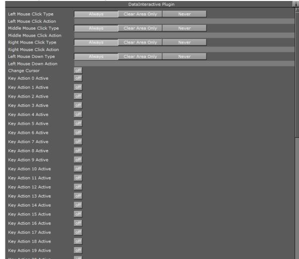
· When using DataInteractive plugin, DataManipulate and DataClick cannot be used.
