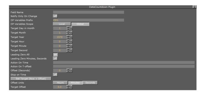
• **DP variables Prefix:** Variable prefix is added to a set of fixed names, based on time scale, for different time variables. The prefix is used to distinguish one set of time parameters from the other. The default prefix is CD1. For example, if Prefix is set to DDay, the corresponding variables are:
