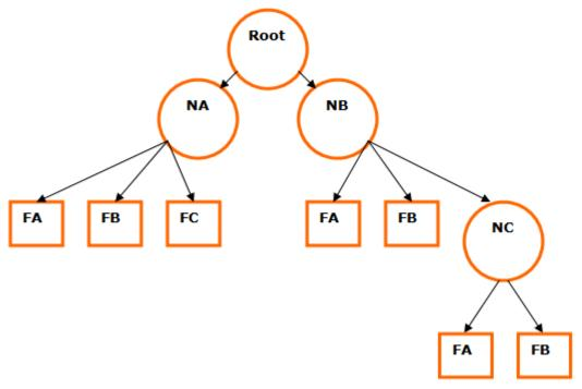
In this example NB has a child node called NC. To set data to the field FB under NC the following command is sent:
