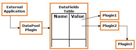
DataPool implements a table of DataFields. Each DataField has a unique name by which it is accessed, a value (data) and a list of data changes handlers. The handlers are implemented as plugins in Viz, where each plugin affects specific parameters of a container in Viz. The plugin instances are registered to DataFields when attached to a container in the scene. The plugin modifies the container parameters when the value of the DataField changes. It doesn't do anything unless it is called.
